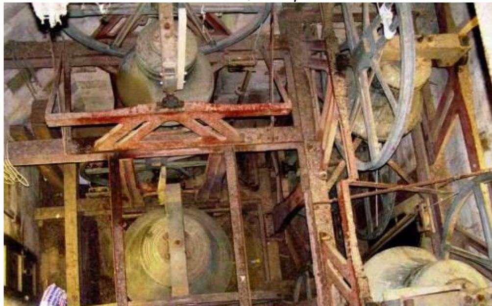
ball races off and cleaned them with white spirit before re-greasing and refitting them. We removed all the pulleys, and Graham took them to the works to exchange all the old oak pulleys for modern ones with ball bearings. Whites also rebushed the front five clappers.
